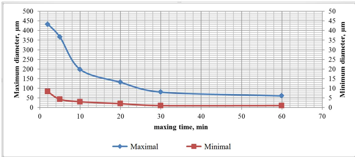
Figure 2 - The dependence of the globules diameters (maximum and minimum) from the mixing time
