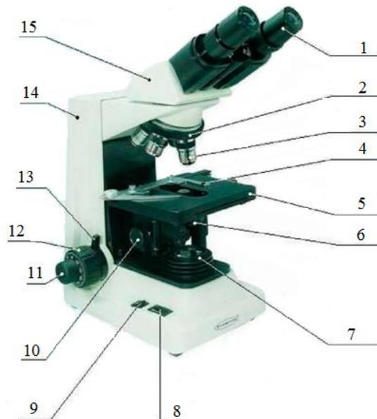
*1-ocular; 2-revolving arrangement; 3-lens; 4-substage; 5-object table; 6-condenser; 7-illuminating lens mount; 8-lamp voltage regulator; 9-microscope toggle on / off; 10-handle for moving the condenser up and down; 11-fine focus handle; 12-coarse focus handle; 13-restraint table displacement handle; 14- tripod; 15-binocular adjustment.*
